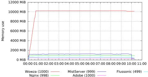
No surprises here, keeping the Q1 results in mind. Wowza still uses roughly 10GiB of memory for 1000 clients, while MistServer and Nginx use roughly 1GiB. Adobe and Flussonic manage even less, with Adobe taking the memory-efficiency crown.
