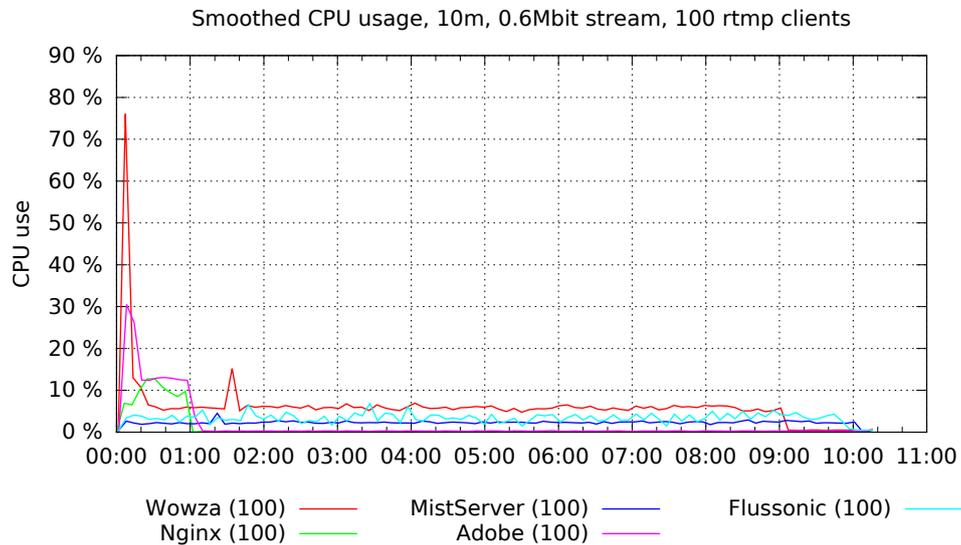
This is the CPU usage for a ten minute test of 100 clients, for all tested applications. **Less is better. The number between parenthesis is the count of successful clients.**
