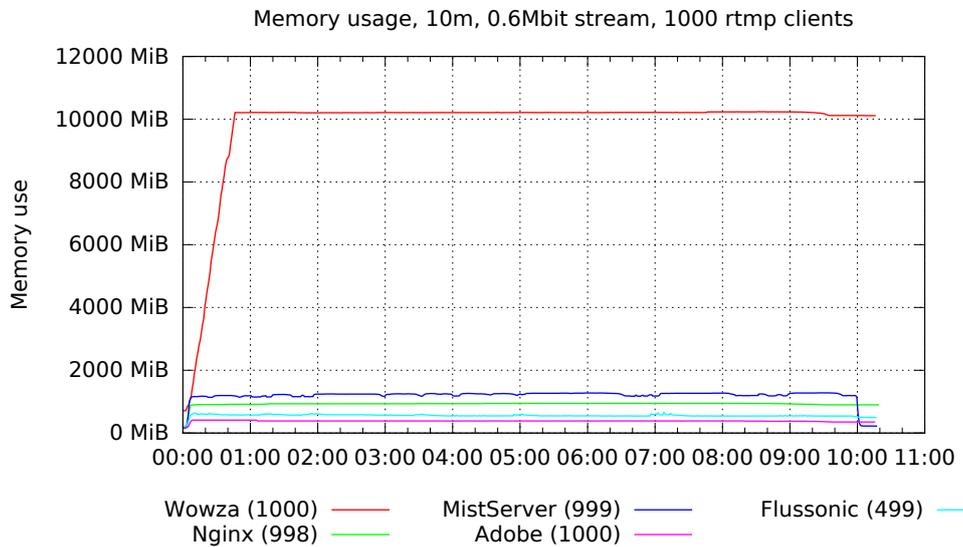
No surprises here, keeping the Q1 results in mind. Wowza still uses roughly 10GiB of memory for 1000 clients, while MistServer and Nginx use roughly 1GiB. Adobe and Flussonic manage even less, with Adobe taking the memory-efficiency crown.
