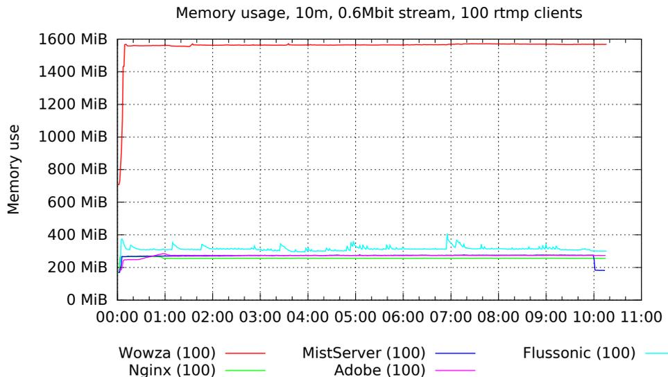
Again, **less is better**, and the number between parenthesis is the count of successful clients. In this case, Wowza has not improved but actually is using roughly 200 MiB more memory than in the Q1 results. The others haven't changed much, staying at approximately 300 MiB for 100 clients.
